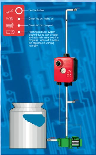
In case the pump switches on/off repeatedly, due to the system leakages, it will be necessary to install, after SuperSimplex, a pressure tank of 2-8 litres capacity.
